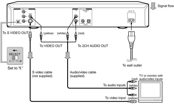
If the TV has an S video input, connect the DVD player with an S video cable. When using an S video cable, do not connect the yellow video cable.
